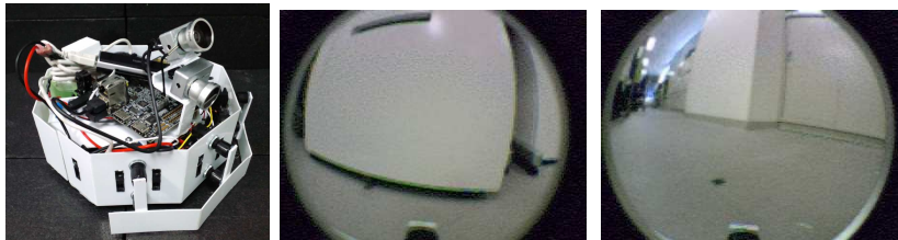
Fig. 1. (Left) Our autonomous mobile robot. (Middle) Example of images taken by the robot. Note the thin green line under the shelf. (Right) Another example. Note the blue light at upper left window, which was unnoticed with more than 7500 images taken in this run.
